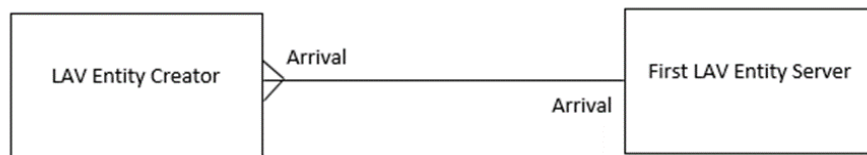
Figure 11. Listener Diagram Depicting Entities being Passed from the LAV Entity Creator Class to the First LAV Entity Server Instance
