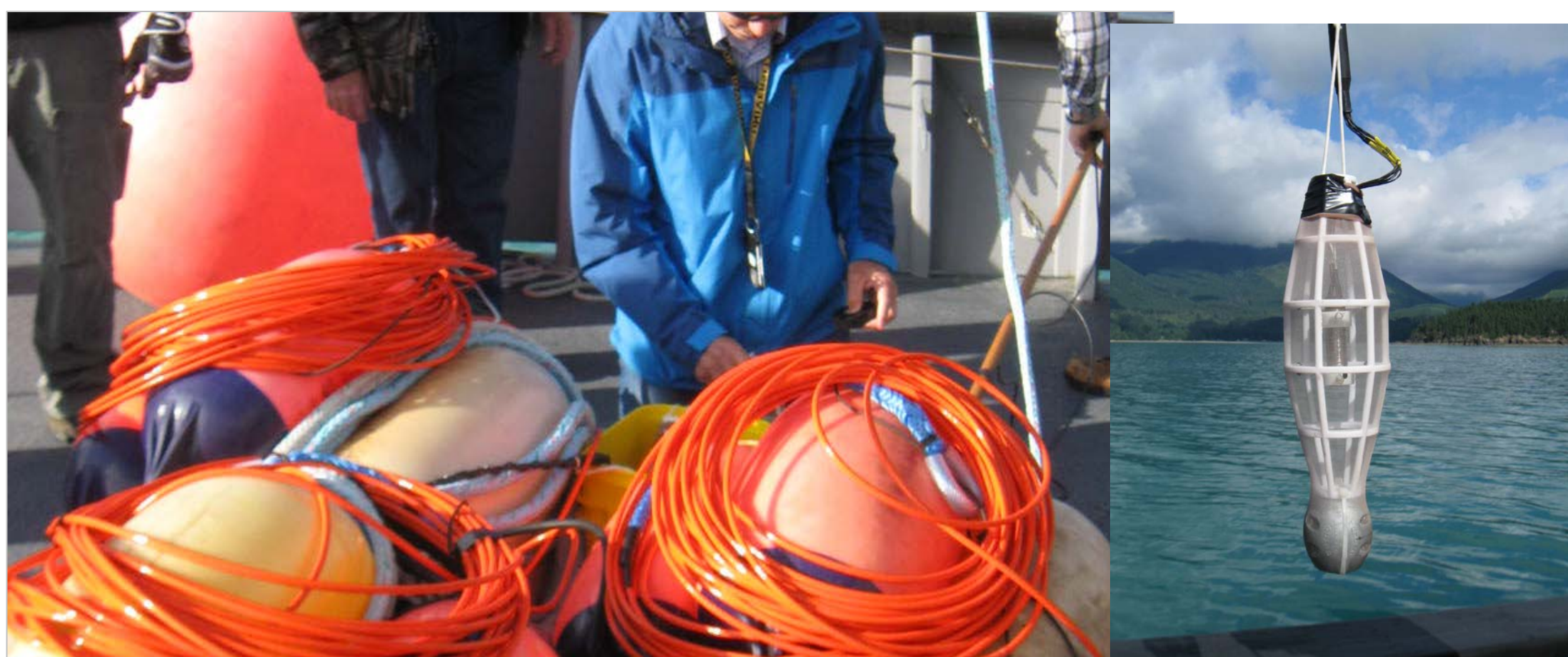
Drifting buoy systems (left) and tethered vector sensor suspended in mount (right) being prepared for deployment in Dabob Bay, Sept 2017.
