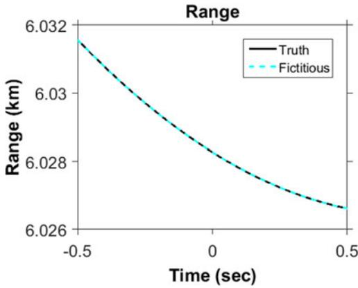
Fig. 6. Range values for the true and fictitious target motions are identical to the precision of the machine computations.
