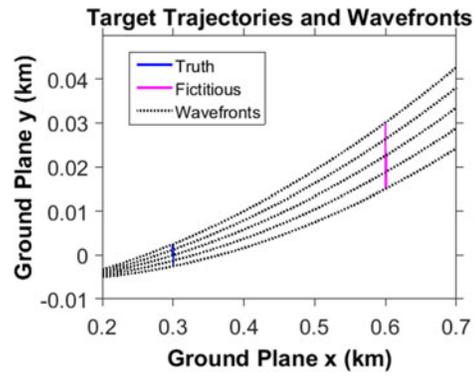
Fig. 8. Zoomed image of the true and the second fictitious target trajectories, including five circular wavefronts evaluated at the  $\{0, 1/4, 1/2, 3/4, 1\}$  fractions of the full synthetic aperture.
