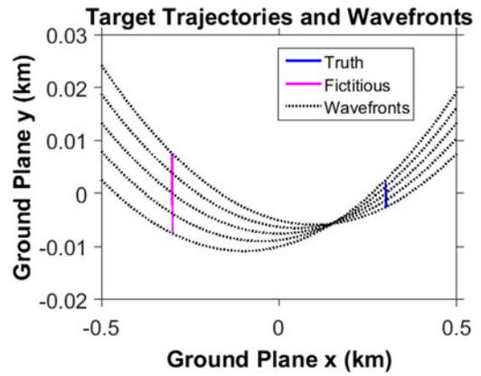
Fig. 3. Zoomed image of the true and first fictitious target trajectories, including five circular wavefronts at the  $\{0, 0.25, 0.5, 0.75, 1\}$  fractions of the full synthetic aperture.
