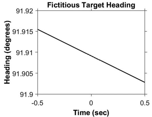
Fig. 5. Heading of the first fictitious target varies by less than  $0.1^\circ$  over the full SAR collection duration.
