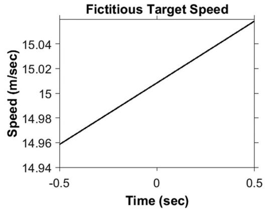
Fig. 4. Speed of the first fictitious target varies by less than 1% over the full SAR collection duration.
