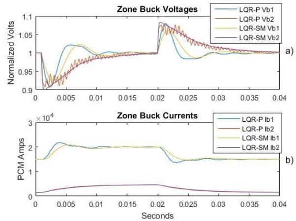
Figure 7 – Zone Normalized Volts and Currents from Buck Converters
