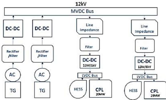
Figure 2 - Simplified Illustration of Shipboard MVDC Distribution System
