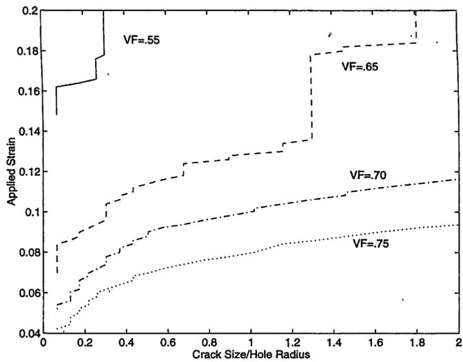
Fig. 7 Normalized crack size versus applied uniform strain for different particle volume fractions
