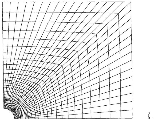
Fig. 6 Finite element mesh with a 0.25-in. hole
