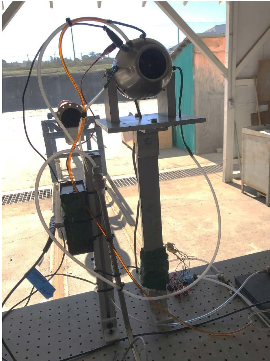
Figure 19. The hydrogen tubing from the steel line into the engine
