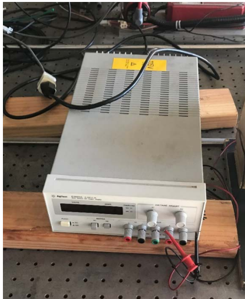
Figure 23. Oil pump power supply connected to relay to remotely start the pump
