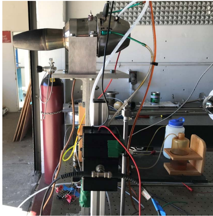
Figure 21. The engine apparatus mounted in the test cell
