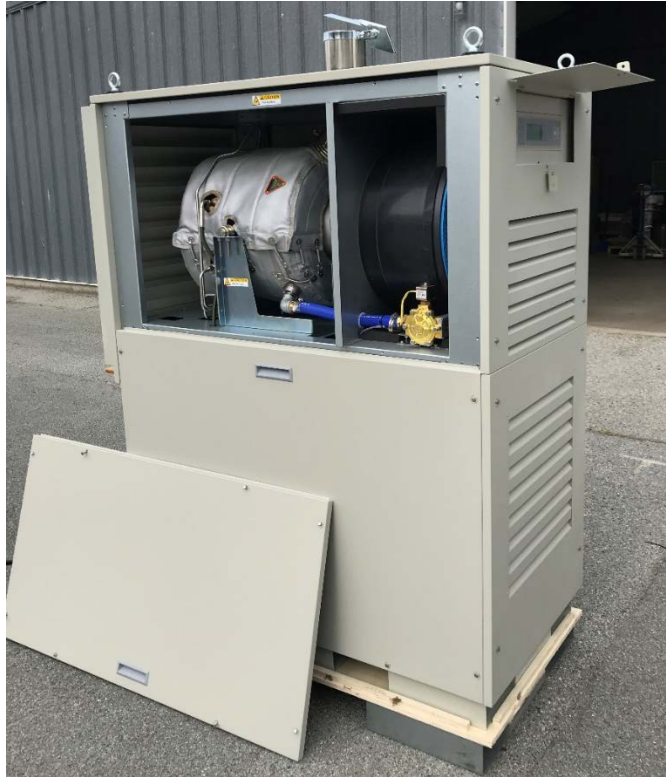
Figure 33. The C30 Capstone engine successfully run off propane gas
