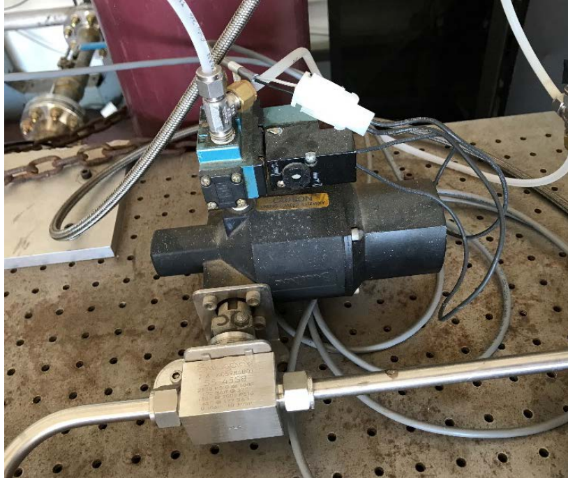
Figure 17. Hydrogen ball valve to control hydrogen flow
