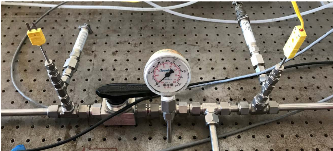
Figure 18. Hydrogen supply valve with associated pressure gauge to read the pressure supplied into the engine
