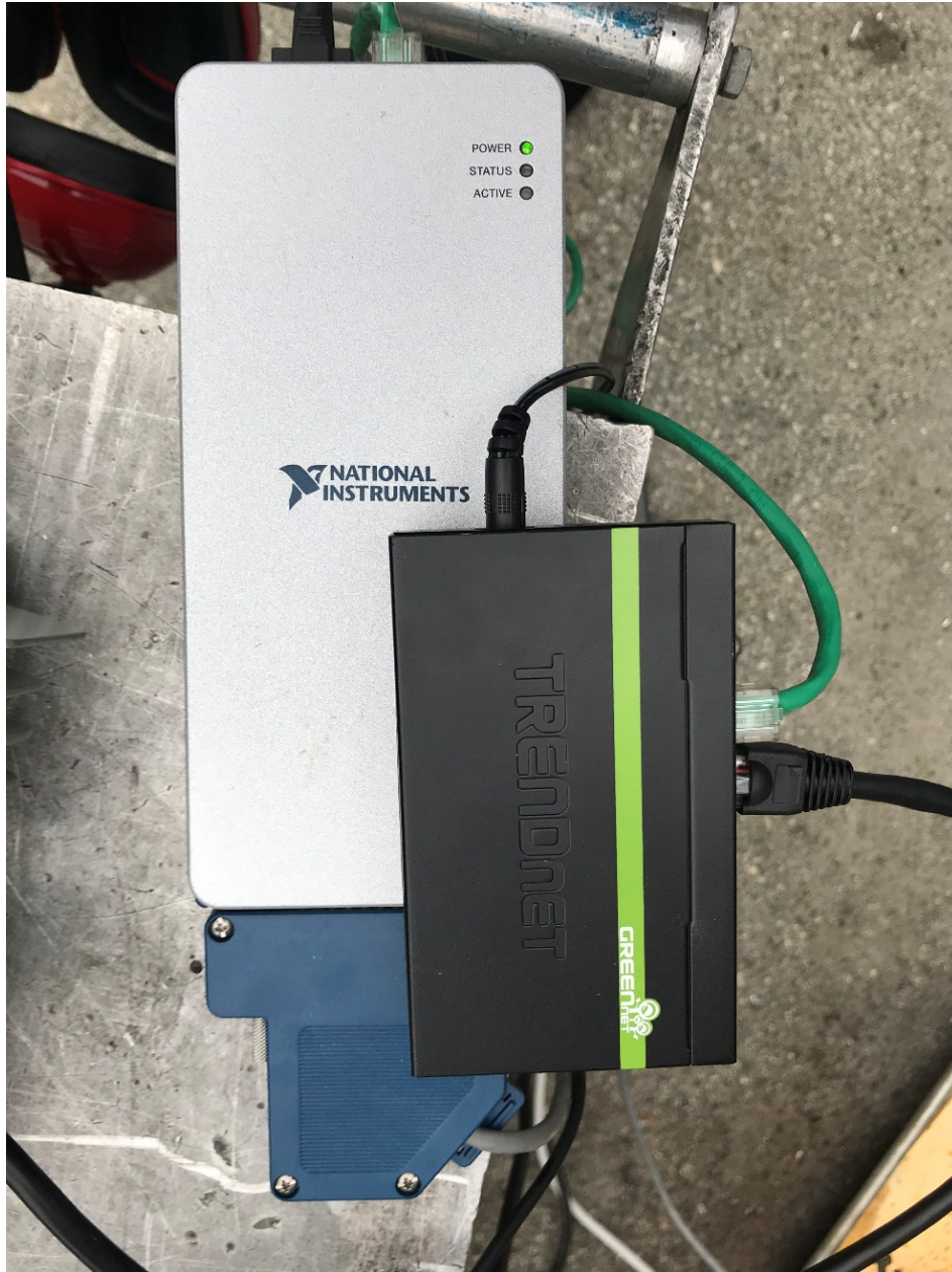
Figure 14. The National Instruments strain gauge measured the voltage across the full Wheatstone bridge
