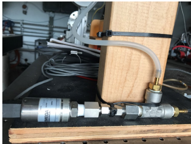
Figure 25. Pressure transducer connecting the relay, a pressure gauge, and to the engine piping
