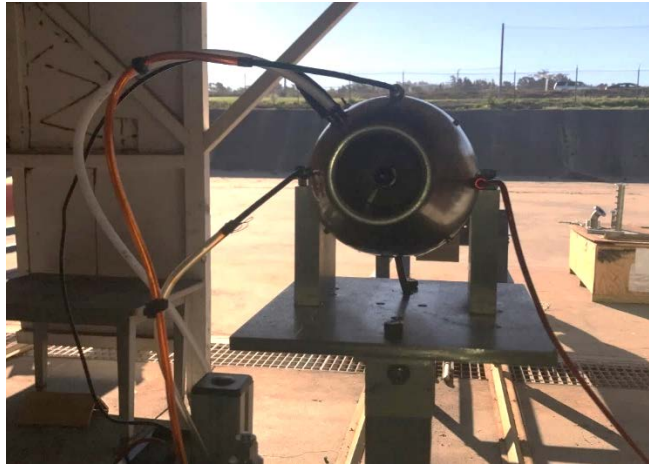
Figure 24. Piping configuration into the engine apparatus
