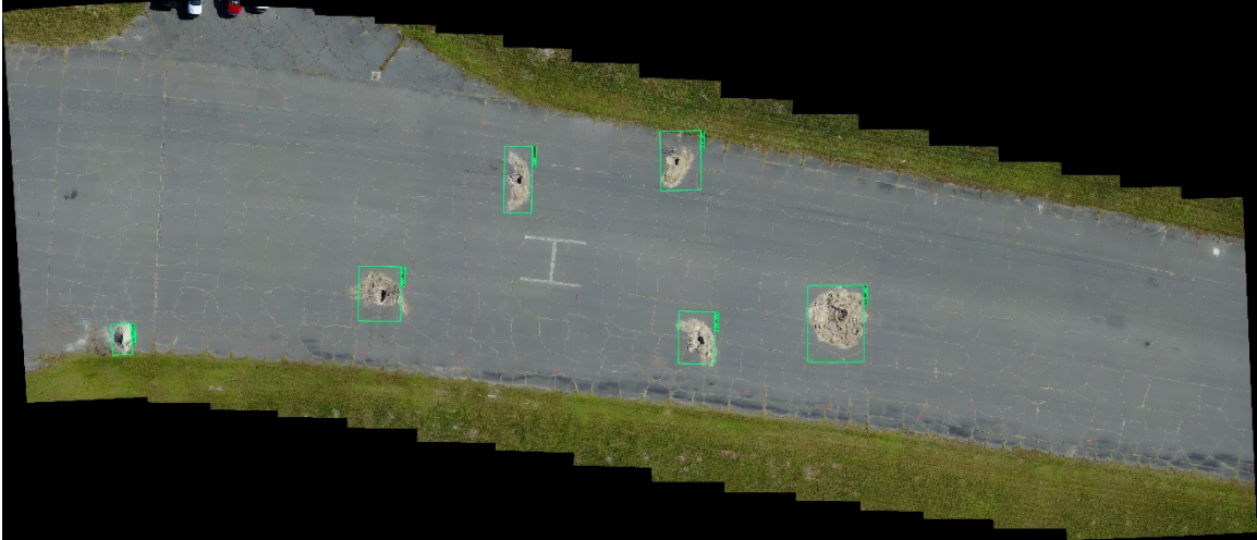
Figure 26. Example mosaic of a runway produced from a series of images taken from a UAV with automatic damage detection.
