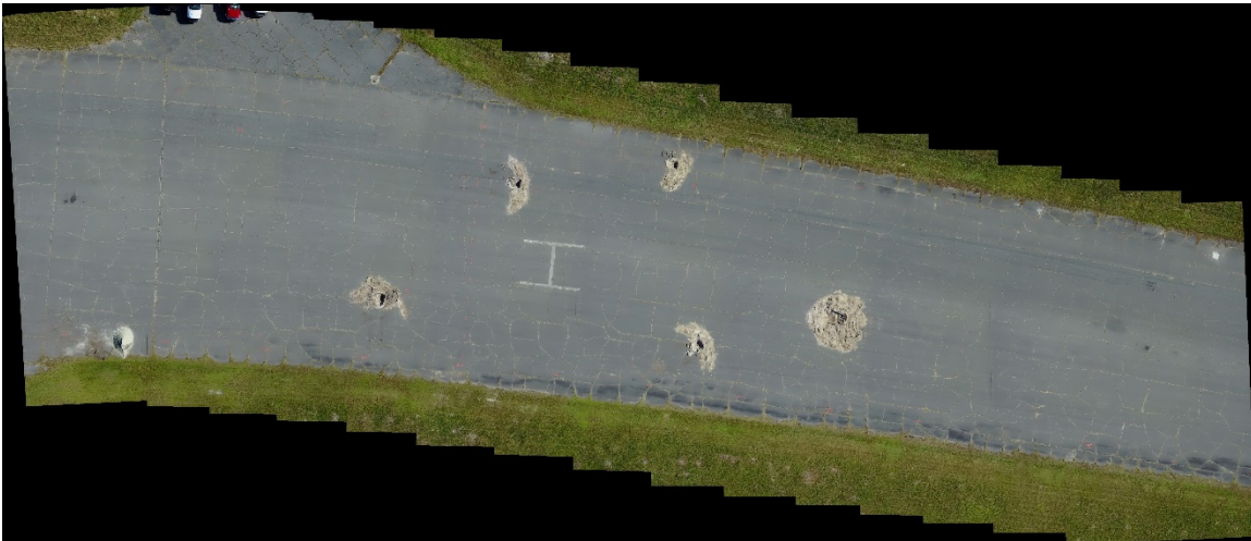
Figure 25. Example mosaic of a runway produced from a series of images taken from a UAV.
