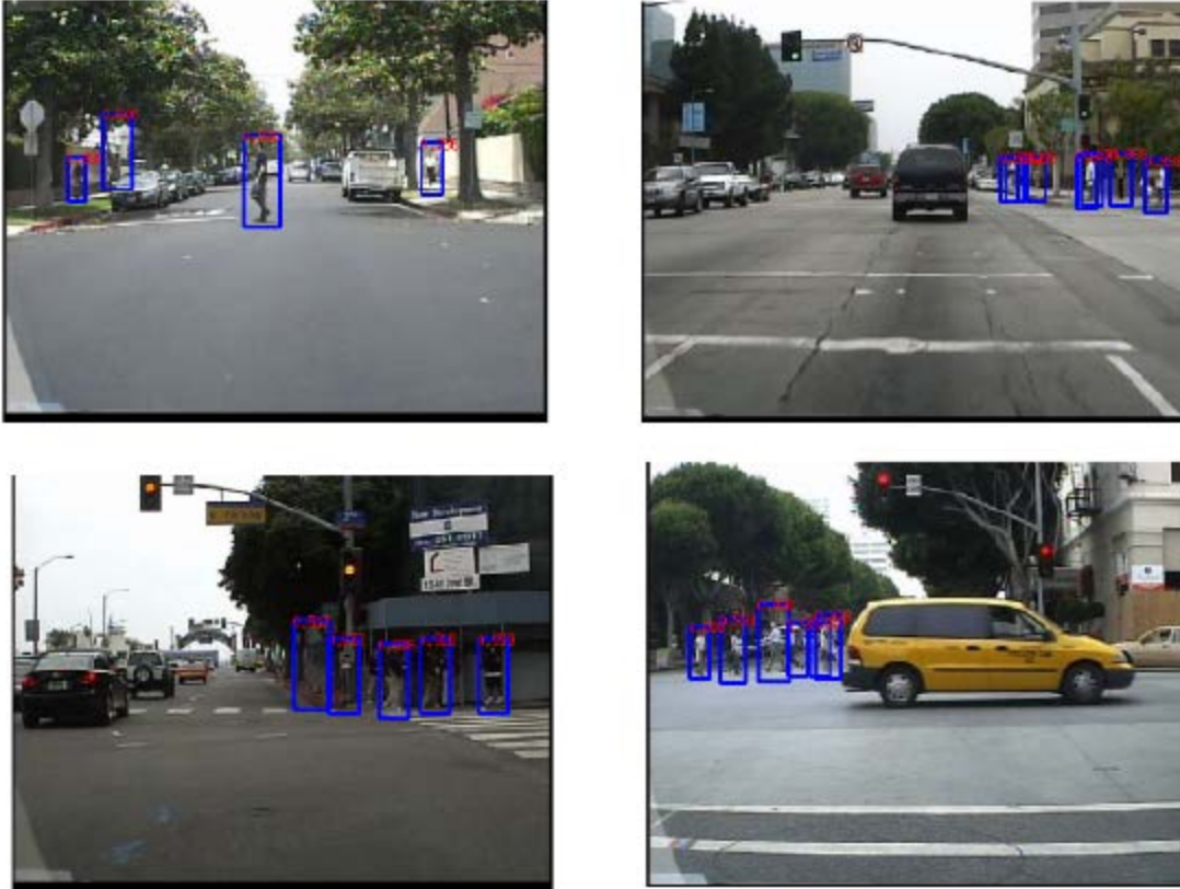
Figure 11. Examples of detecting pedestrians using a trained neural network. Source: Angelova et al. (2015).
