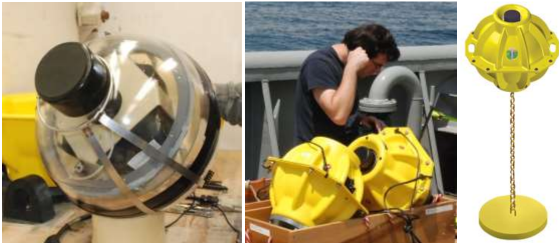
Figure 73. Modem-recorders are housed in pressure-tolerant glass spheres for deployment at depth. Received acoustic signals are digitally recorded to removable SD cards for later analysis.
