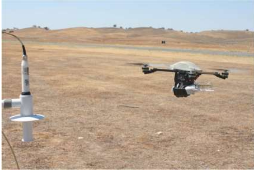
Figure 58. InstantEye UAV with Vaisala RS-92 radiosonde attached on bottom. The UAV is hovering next to a temperature/humidity sensor (left side) to verify and validate the UAV/radiosonde measurements
