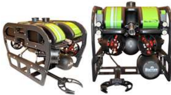
Figure 48. The SeaBotix vLBV300 ROV platform
