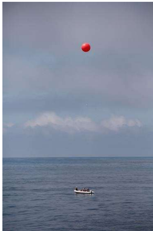
Figure 55. Tethersonde operations from a small boat during TW13. A radiosonde (not visible) is attached below the balloon which is raised and lowered several times from 1 m to 200 m elevation. These measurements were a proxy for mini quad rotor UAV sampling of the atmosphere.
