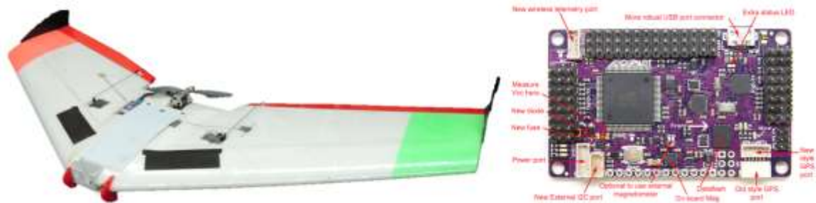
Figure 44. Prototype NPS ARSENL UAV designs integrating low-cost Ritewing ZephyrII RC aircraft platform (left) and the open-source APM autopilot (right) 6
