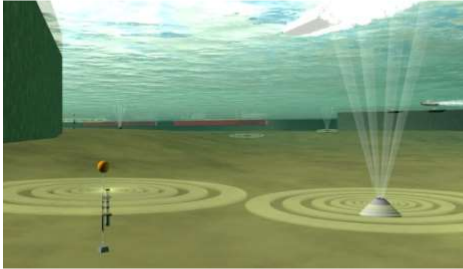
Figure 74. Maritime In Situ Sensing Inter-Operable Networks (MISSION) deliver near-real-time data from distributed underwater sensor stations.
