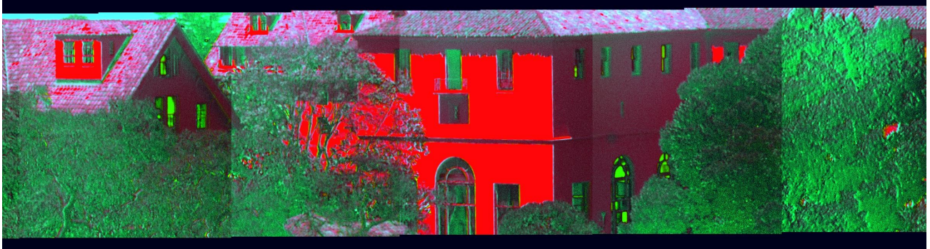
Figure 5. An RGB image with the s_0 image mapped to Red, DOLP mapped to Green, and s_1 mapped to Blue.
