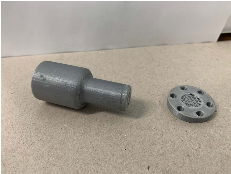
Figure 21. Failed PLA Coupling Device
