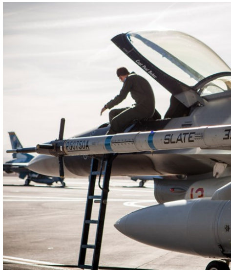
Figure 1. USAF F-16 with the SLATE 5G -ATW pod deployed at Nellis AFB, NV. Source: Magnuson (2019).
