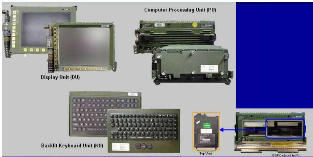
Figure 8. BFT components. Source: MCCSSS (2016, p. 7).
