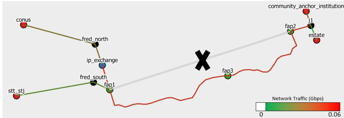
Figure 3.14. Layer-1 Traffic Assignment in Simple Model, One Edge Destroyed. Aggregate traffic over layer-1 edges with edge (‘fap1’, ‘fap2’) destroyed. The black ‘X’ represents a fiber optic cable cut. White lines indicate no traffic flow. Color on edges increases from green to red as the amount of traffic flow over the layer-1 edge increases. Traffic flow has been re-routed over an alternate layer-2 route.
