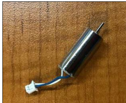
Figure 20. XK Innovation 0720 Brushed Motor (Tail Motor).
