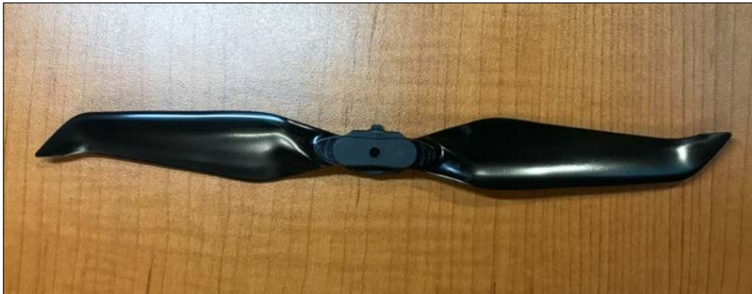
Figure 17. Master Airscrew Stealth 8743F Propeller.
