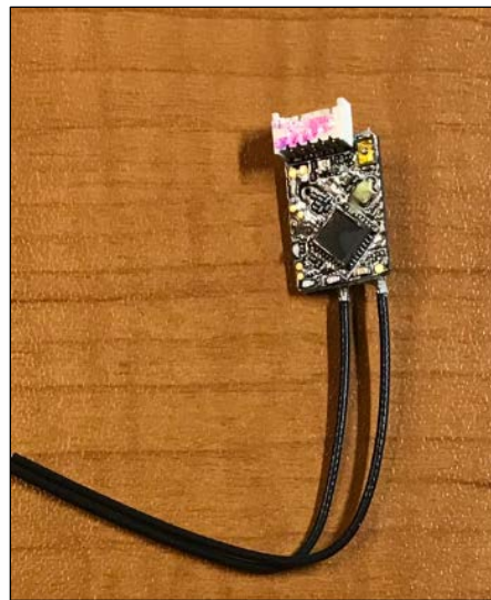
Figure 26. FrSky R-XSR 2.4 GHz 16 Channel ACCST Micro Receiver.
