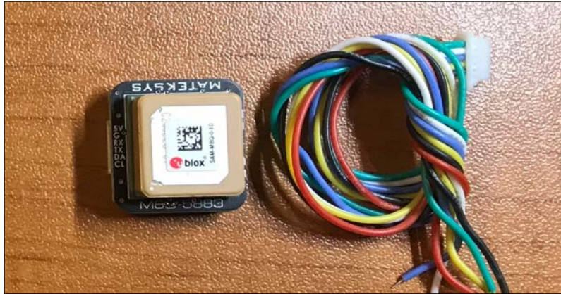
Figure 30. Mateksys M8Q-5883 GPS Module w/Compass.
