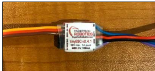
Figure 23. FingerTech tinyESC V2 (for the Tail Motor).
