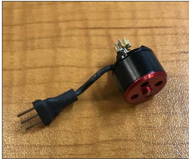
Figure 19. XK Innovation 1106–11,000 KV Brushless Motor (Main Motor).
