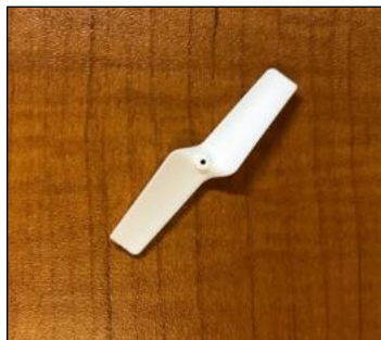
Figure 18. XK Innovations K120 Helicopter Tail Propeller.
