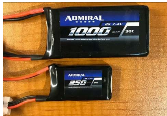
Figure 21. Admiral 250 mAh 2S 30C LiPo Battery.
