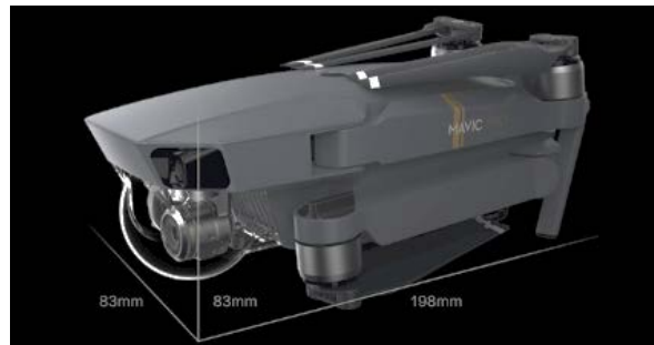
Figure 6. Folded DJI Mavic Pro with Dimensions. 50
