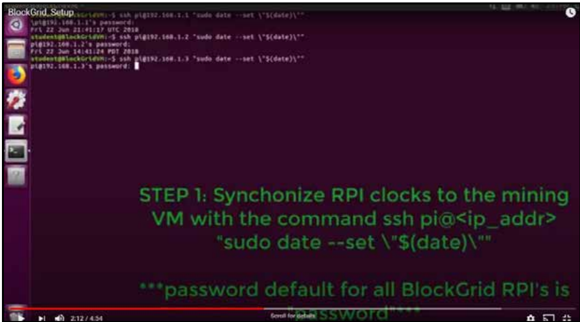
Figure 34. Screenshot from Prototype Setup Instructional Video Showing How to Synchronize RPI clocks.
