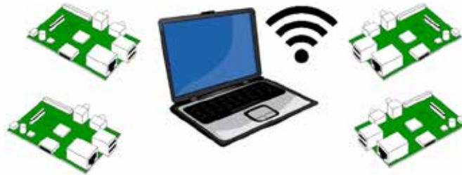
Figure 12. Networking Configuration with WLAN through a Software Router.
