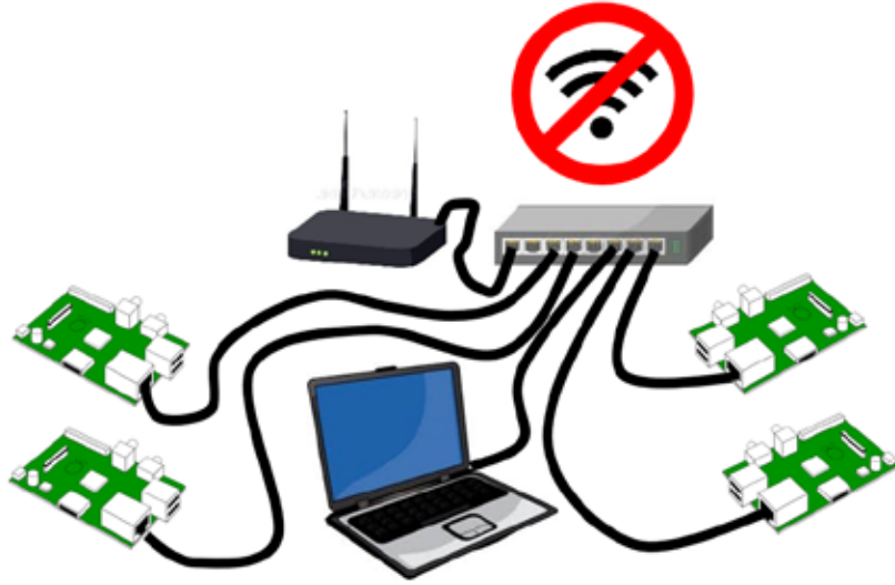
Figure 15. Networking Configuration with an Internal Ethernet Connection.
