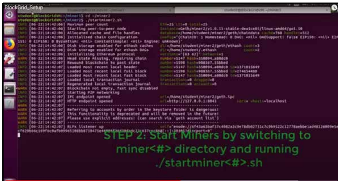
Figure 35. Screenshot from Prototype Setup Instructional Video Showing How to Start Miner Nodes.
