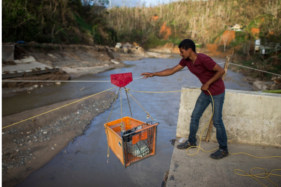
Figure 1. Pulley System to Span the Río Viví. 166
