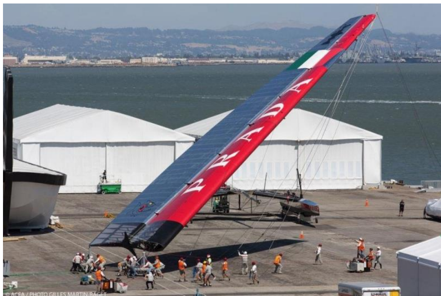
Figure 26 AC72 mast stepping operation. Source: [12].
