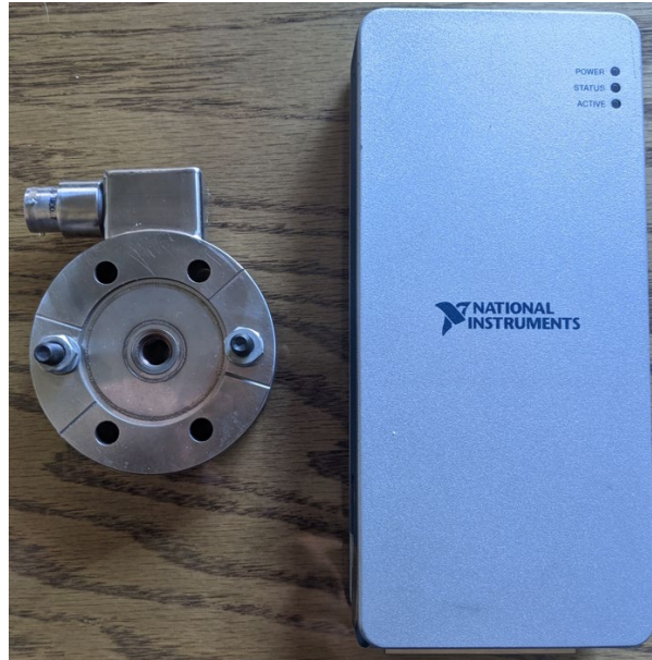
Figure 6 Honeywell loadcell (left) and National Instruments data acquisition module (right)
