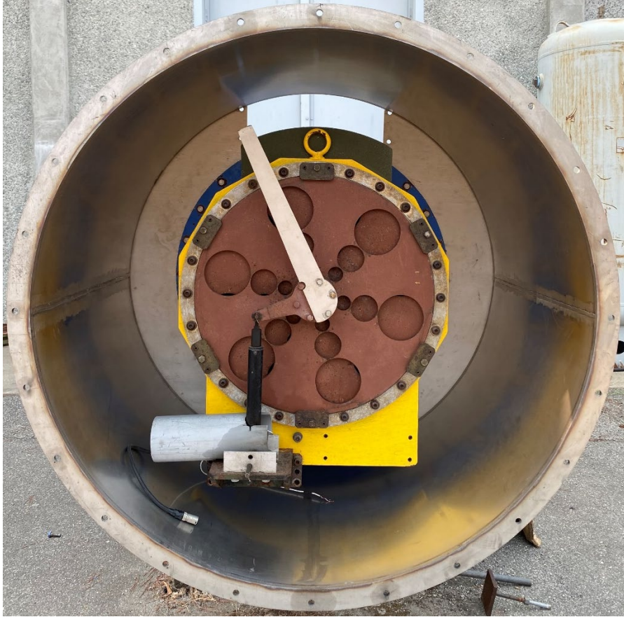
Figure 4. Throttle surrounded by the throttle casing, to which the bell mouth would be attached.
