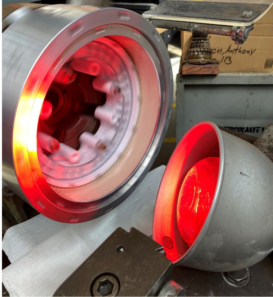
Figure 53. Epoxy Pouring for Internal Passage Treatment
