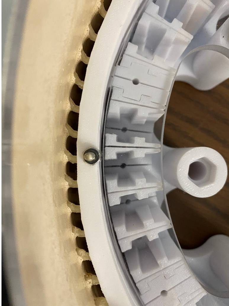
Figure 55. Internal Passage Casing Treatment Immediately After Epoxy Cured
