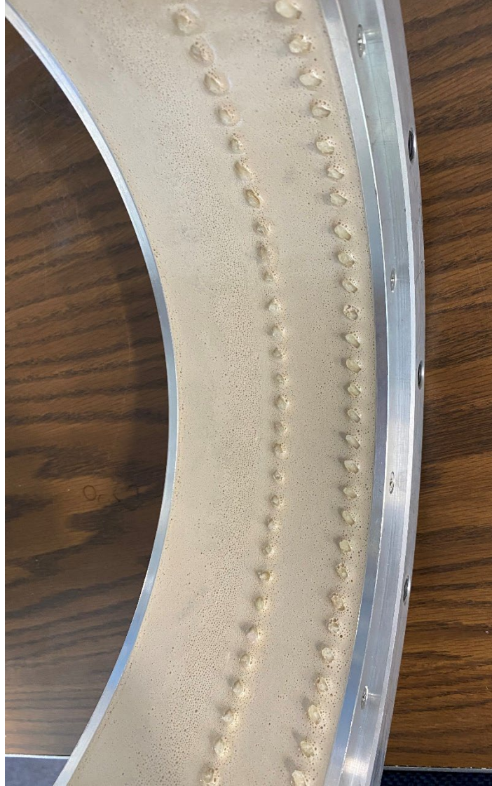
Figure 56. Nearly Completed Internal Passage Casing Treatment
