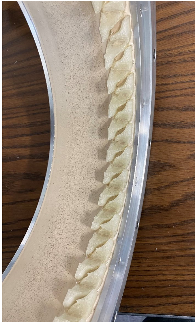
Figure 54. Compressor Casing Surface Treatment Immediately After Mold Base Removal
