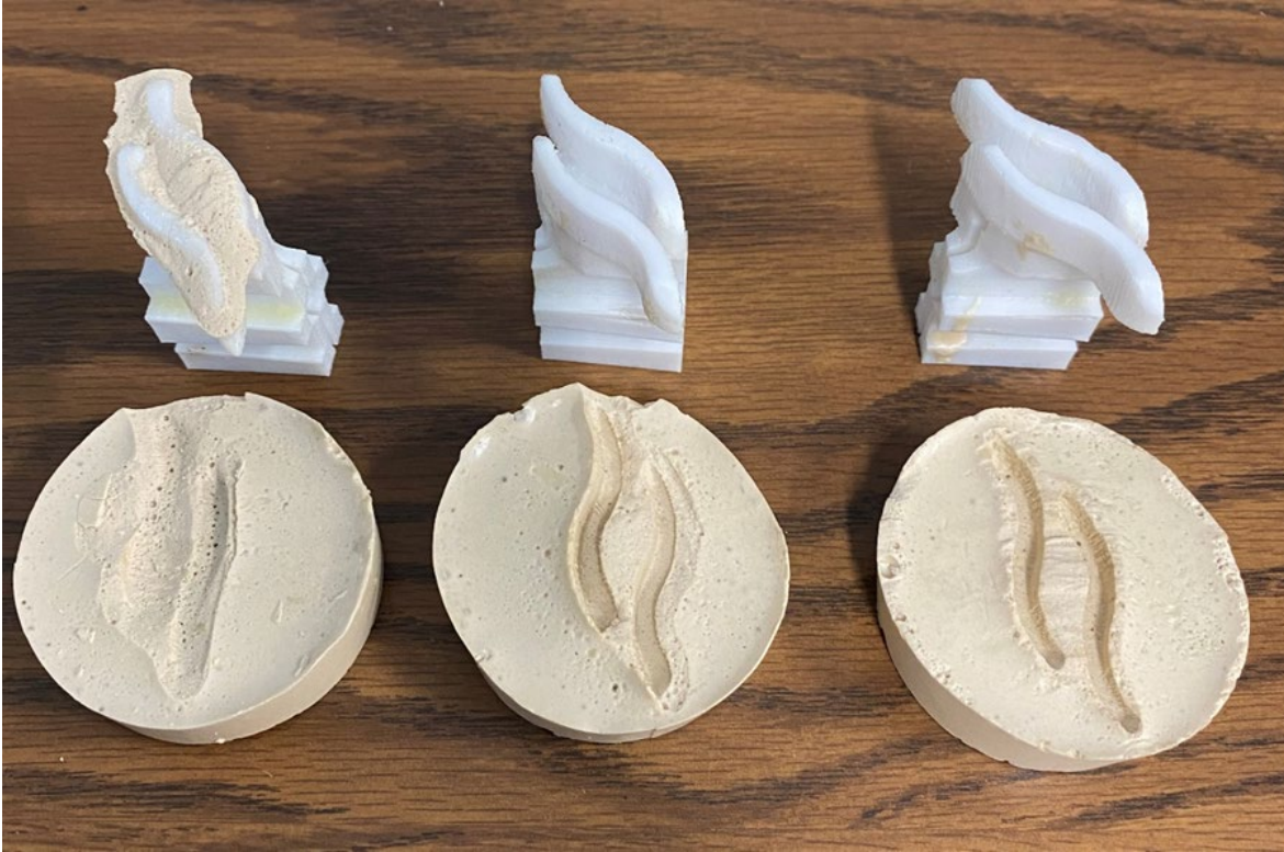
Figure 62. S-Grooves Cast from Epoxy Test
