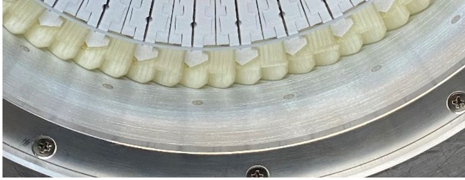
Figure 23. Molds in Place on Casing Zoomed In
