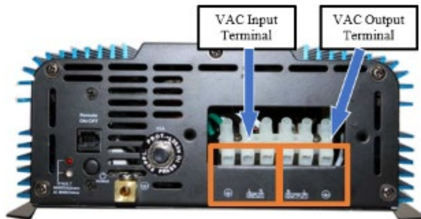
Figure 11. VAC Power Inverter Front View. Adapted from [26].
