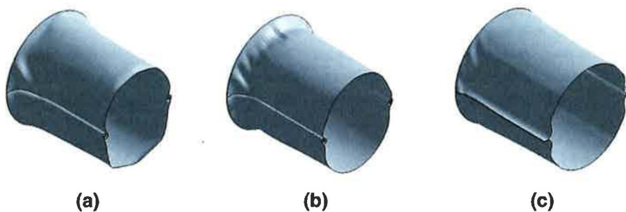
Fig. 54 Dynamically buckled mode shapes for a steel, b aluminum and c composite cylinders without FSI
