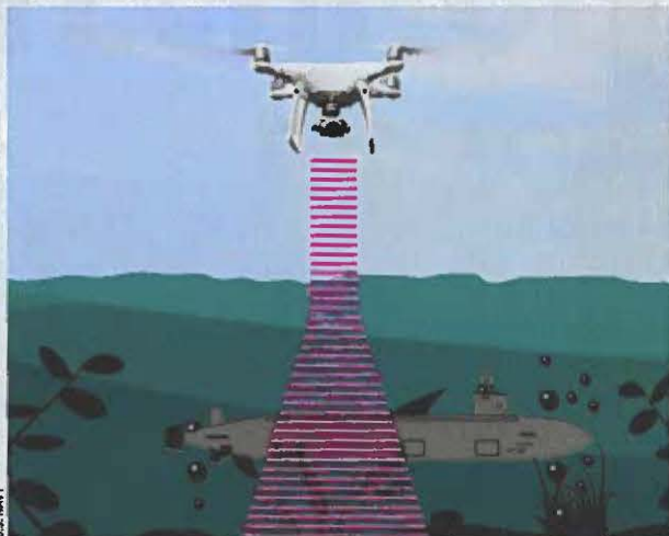
The Office of Naval Research photoacoustic airborne sonar systems (PASS) are low-flying drones that use lasers to vaporize water near the surface to generate underwater sound, which propagates like a sonar ping.
