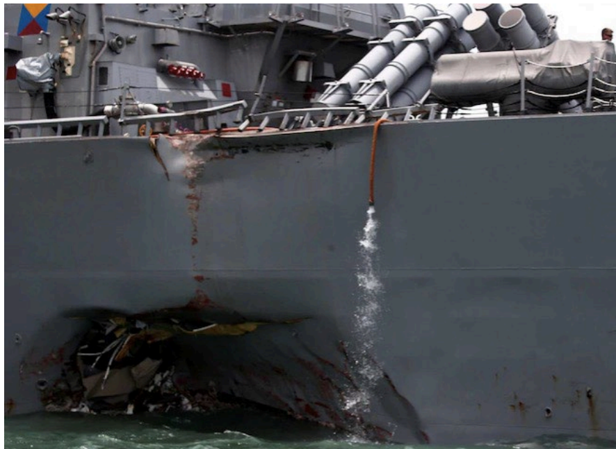
Figure 2. Hull Damage from the USS John S. McCain and Alnic MC Collision. Source: Reuters (2017).
