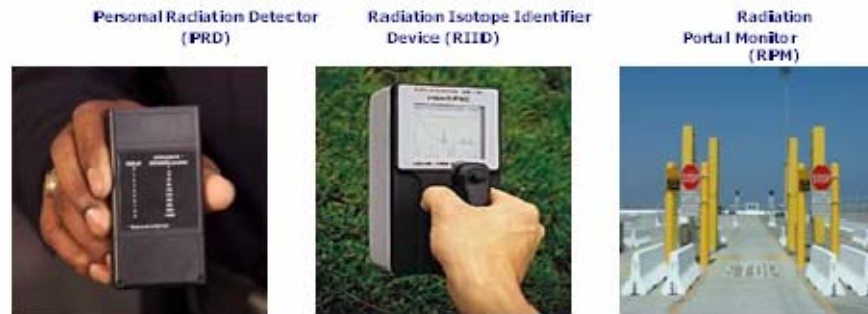
Figure 105: Handheld and Fixed Structure Radiation Detectors [49]
