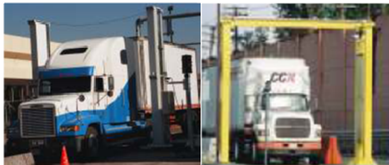
Figure 30. Radiation Portal Monitors
