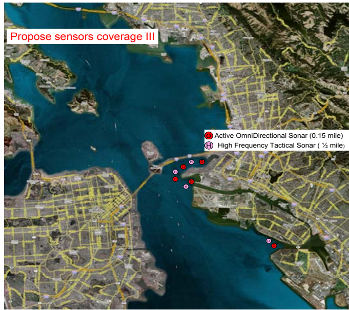
Figure 59. Acoustic Sensor Deployment Plan
