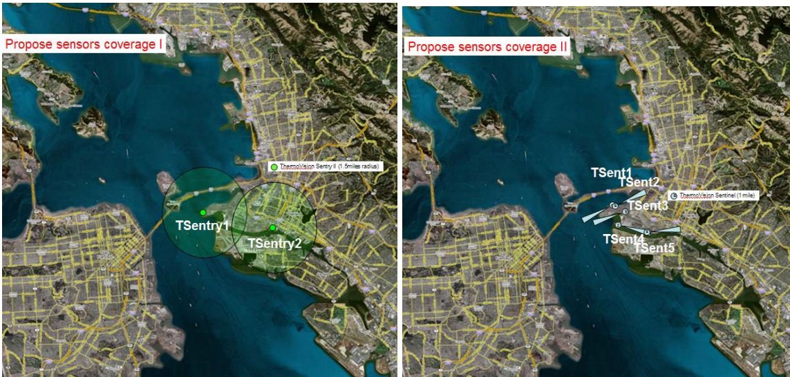
Figure 80. Encoding of Positions and Coverage of the Electro-Optics Sensors
