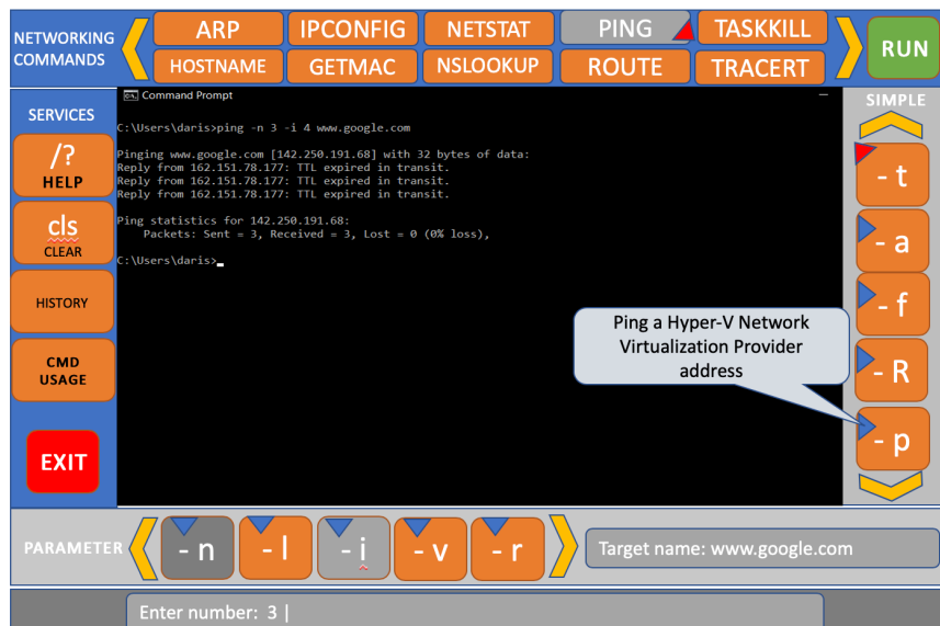
Figure 20. PCCP Mockup #3: Showing InputField to replace parameter buttons, and TargetName to input strings
