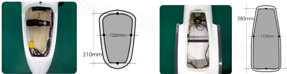
Figure 12. Battery dimensions. Source: [17].
