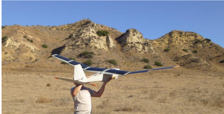
Figure 35. Silicon solar cells on UAV
