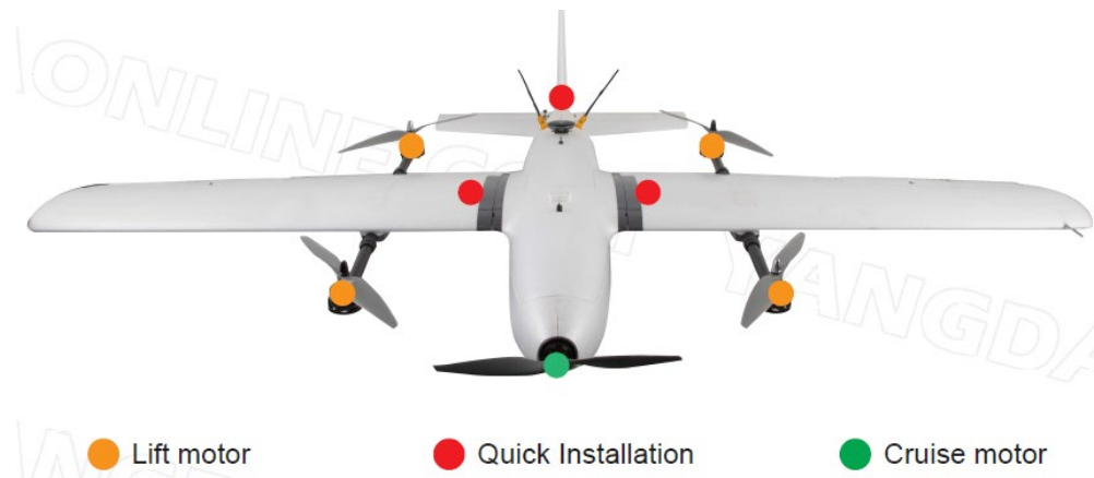
Figure 9. Nimbus Pro VTOL rotors and propellers. Source: [17].
