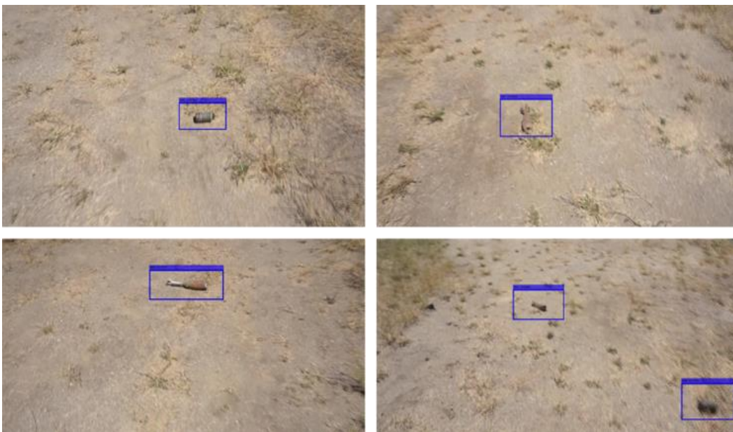
Figure 11. Examples of successful detection of single and multiple UXOs.
