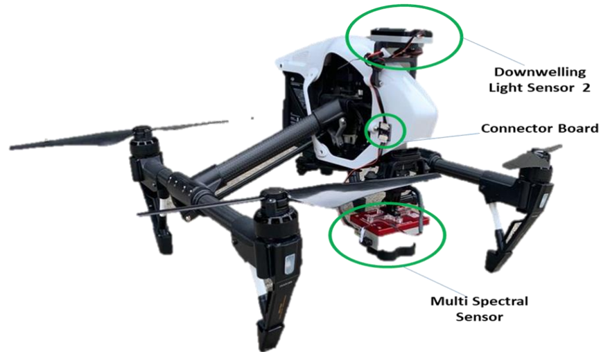
Figure 6. DJI Inspire integrated with a RedEdge-MX sensor.
