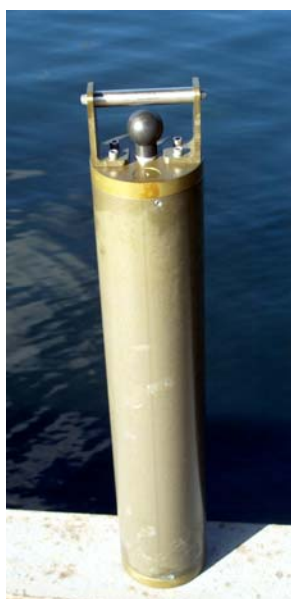
Figure 1. Orfin acoustic data logger
