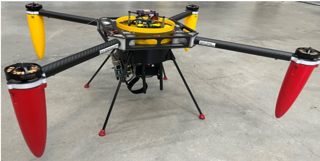
Figure 6.4. Detachable Drone Hijacker attached to its host - The AquaQuad.
