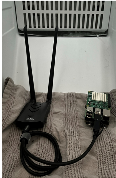
Figure 6.6. Experiment Two Set-up: Sub-Freezing Temperature Testing.
