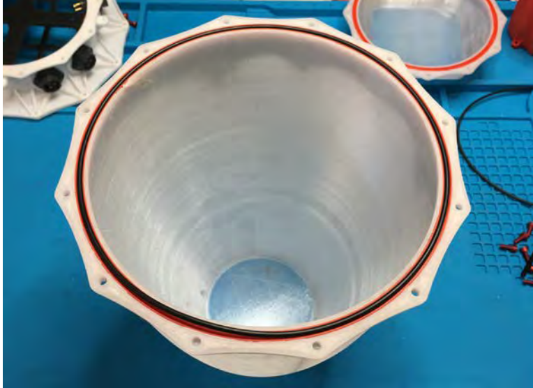
Figure 17. Lower shell of the printed pressure vessel with embedded, printed O-ring seat and O-ring. 3D printed Poly-carbonate with suitable design and printer settings results in water impermeable parts.
