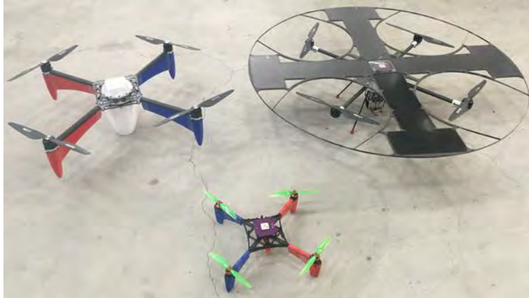
Figure 18. Aqua-Quad prototype models. Rear right: previous generation with solar array mock-up installed. Rear left: current generation with printed pressure vessel and isolated propulsion frame (no array). Front: half size, race-based prototype for low-cost testing of array aerodynamics.
