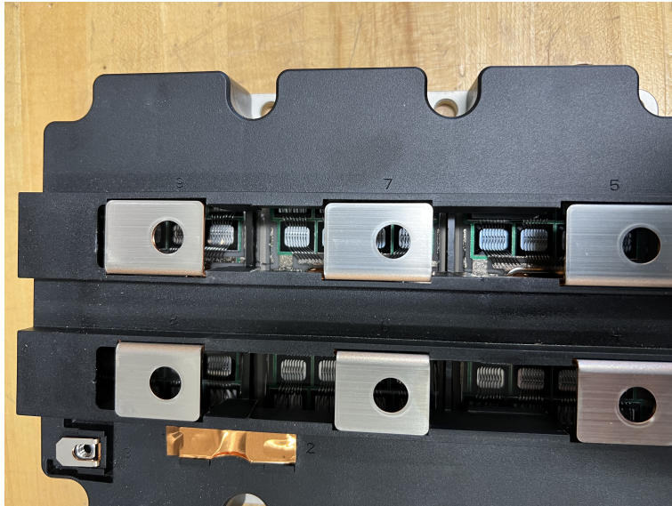
Figure 4.3. IGBT Module with Bus Bars Connection Plate Removed, Chips Exposed
