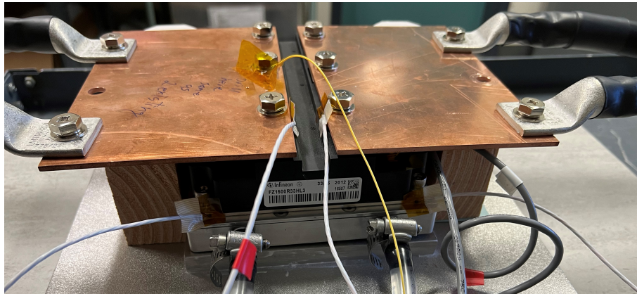
Figure 4.5. Chip Temperature Measurement with Fiber Optic Temperature Probe
