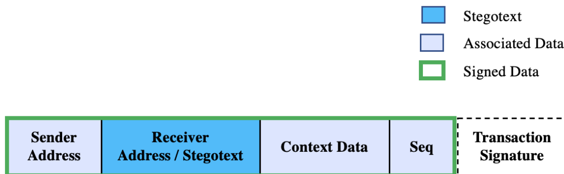
Figure 4.2. Proposed Blockchain-based Transaction Structure with Stegotext
