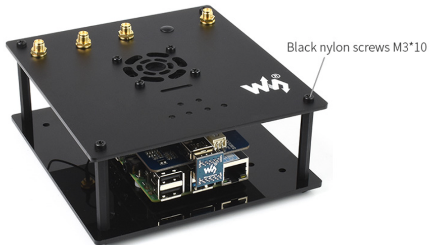
Figure A.5. Installation of 5G Hat and Raspberry Pi: Steps 6-7. Source: [66].
