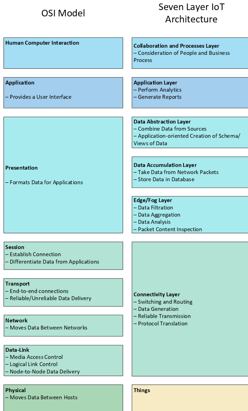
Figure 2. An Evaluation of Iqbal et al.'s (2021) Seven-layer IoT Architecture in Reference to the OSI Model. Adapted from 1-3 OSI Reference Model (2013); Bauer and Patrick (2002); GeeksforGeeks (2022); Iqbal et al. (2021); and Zito (2013).
