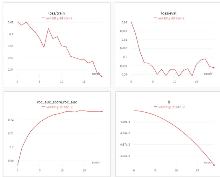
Figure 4.10. Performance results of XLM-T. All metrics are evaluated across 20 epochs. (Top-left) Train loss. (Top-right) Evaluation loss. (Bottom-left) ROC-AUC score. (Bottom-right) Learning rate decay.
