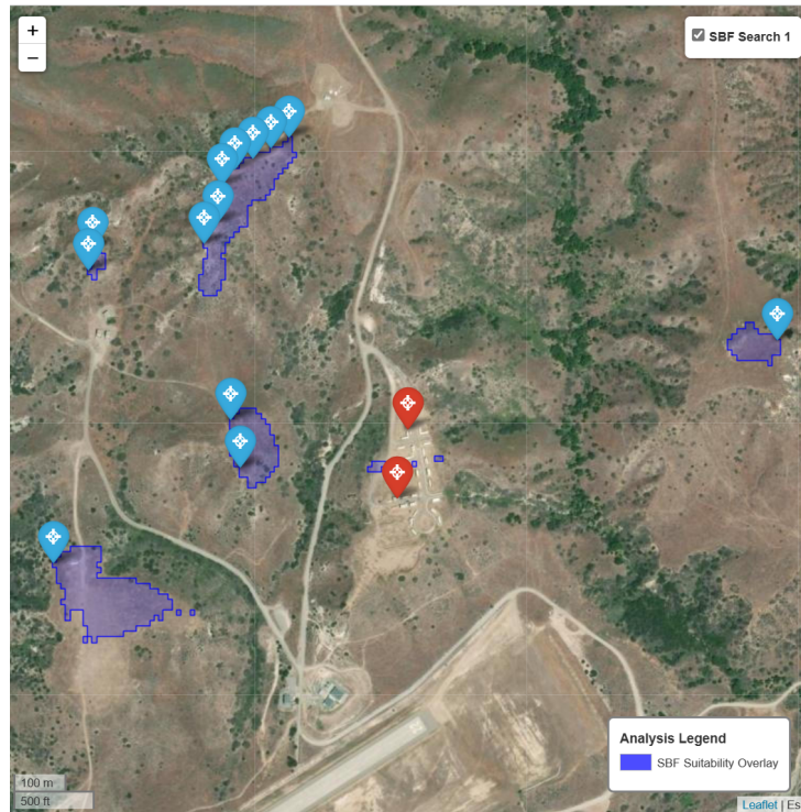
Figure 4.2. The SBF suitability overlay (blue region) delineates the 682 SBF positions that can engage both targets (red markers). We reduce the possible choices down to 13 (blue markers) by imposing three constraints. We specify that the minimum distance to target must be more than 300 meters, a covered position must be within 10 meters, and no position is within 40 meters of another choice position.
