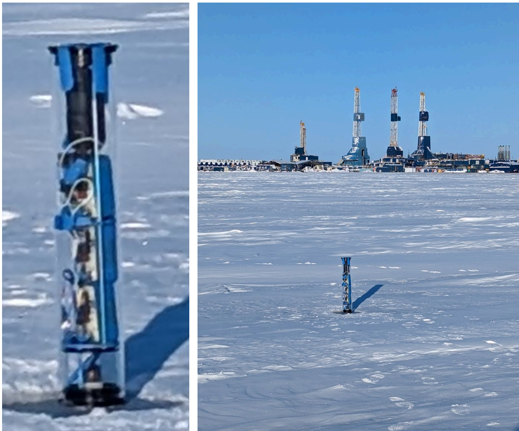
Figure 4: (left) Zoomed view of cryophone comprised of a PCB triaxial accelerometer, three PCB pre-amps, and a Zoom H4N recorder. (right) Cryophone frozen into Lake Colleen.
