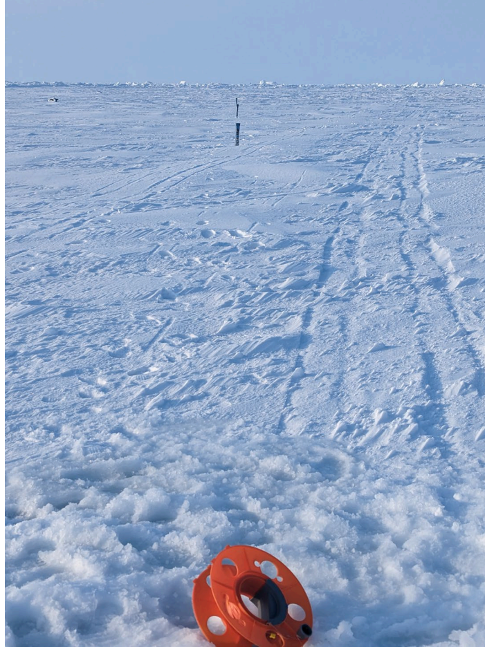
Figure 7: March 10 th : Sea ice floe experiment. VLA (foreground, deployed through a hole under the orange reel), and Cryophone 1, 2, and 3 at 25, 50 and 75 m from VLA hole.
