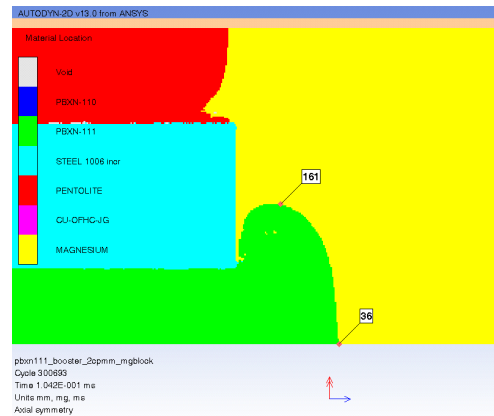
Figure 5.20: Outcome of a cylinder filled with PBXN-111
