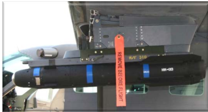
Figure 21. AGM-114K Attached to a Cessna AC-208 144
