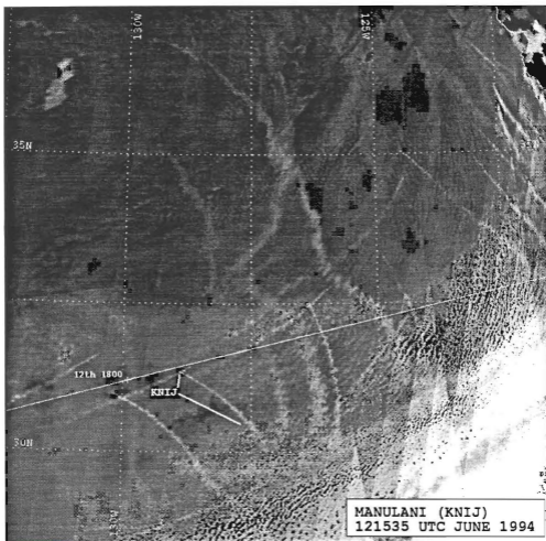
Figure 67. NOAA 12 1535 UTC 12 June 1994 Ch.3 Satellite Imagery Depicting Shiptrack Produced by Container Ship Manulani (KNIJ). Solid line denotes Manulani position history based on synoptic weather reports. Shiptrack location indicated by callsign WCHF.
