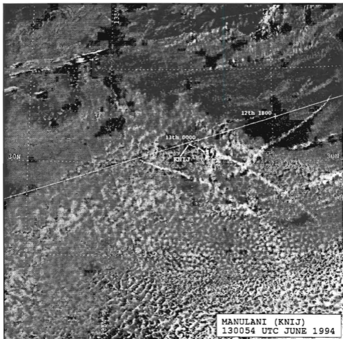
Figure 69. NOAA 11 0054 UTC 13 June 1994 Ch.3 Satellite Imagery Depicting Shiptrack Produced by Container Ship Manulani (KNIJ). Solid line denotes Manulani position history based on synoptic weather reports. Shiptrack location indicated by callsign WCHF.
