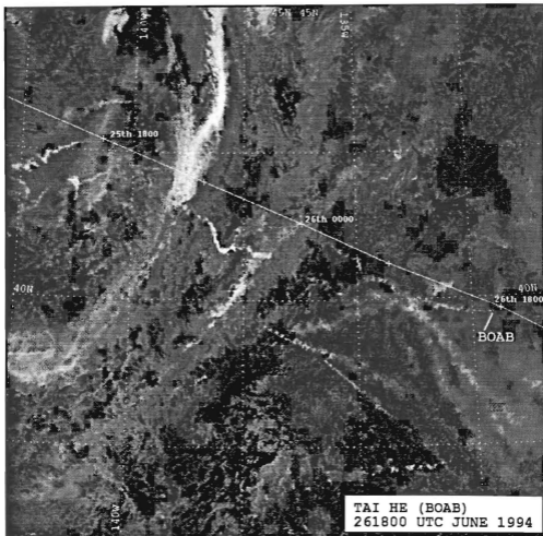
Figure 9. NOAA 09 1800 UTC 26 June 1994 Ch.3 Satellite Imagery Depicting Shiptrack Produced by Container Ship Tai He (BOAB). Solid line denotes Tai He position history based on synoptic weather reports. Shiptrack location indicated by callsign BOAB.
