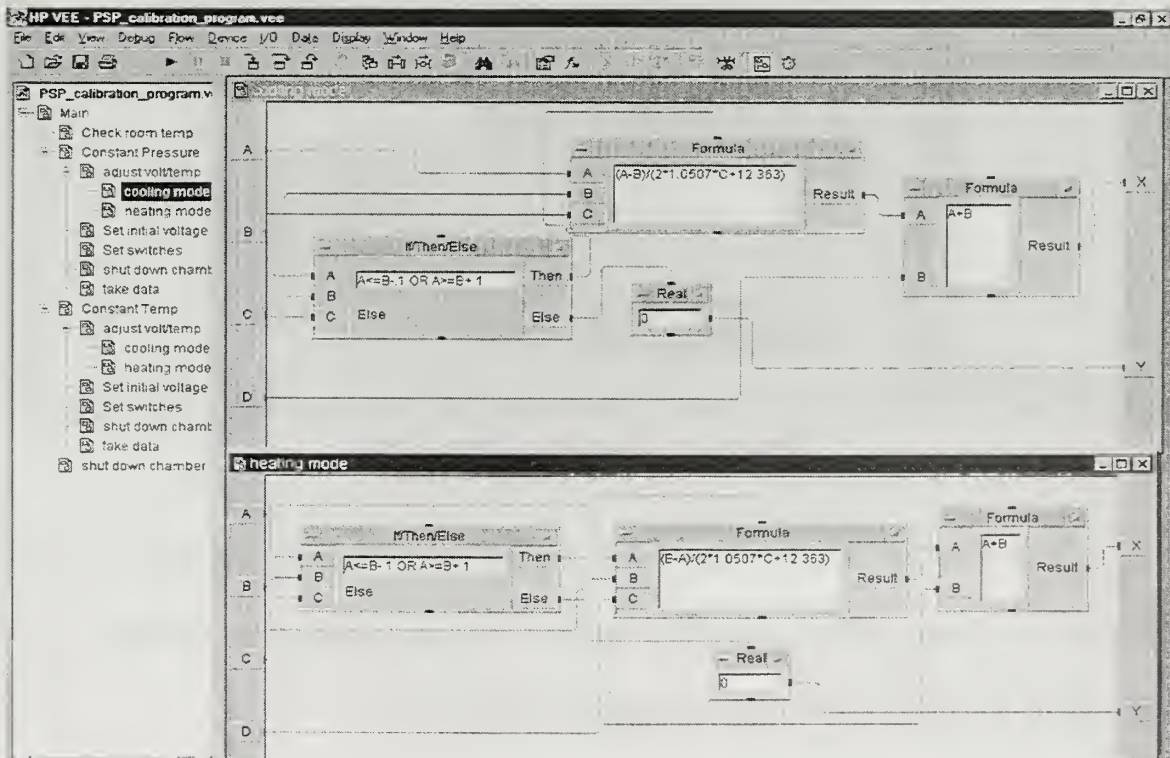
Figure C8. Cooling and Heating Mode Subroutines.
