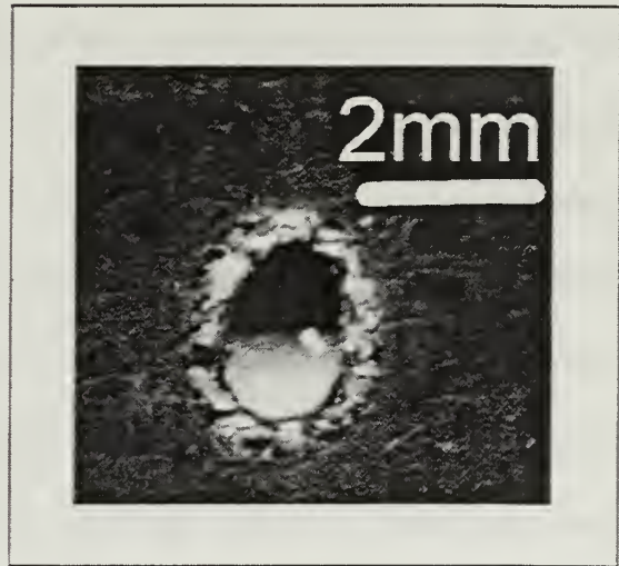
Figure 47. Polyimide exit hole 20. Intensity 10 \text{ kW/cm}^2 , with air. Average Power 500 W. Spot Radius 1.25 mm.
