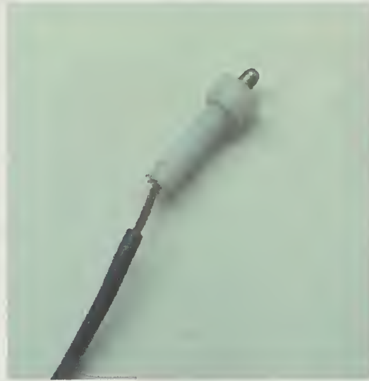
Figure 4. Type J Thermocouple For Sensing Bearing Temperature
