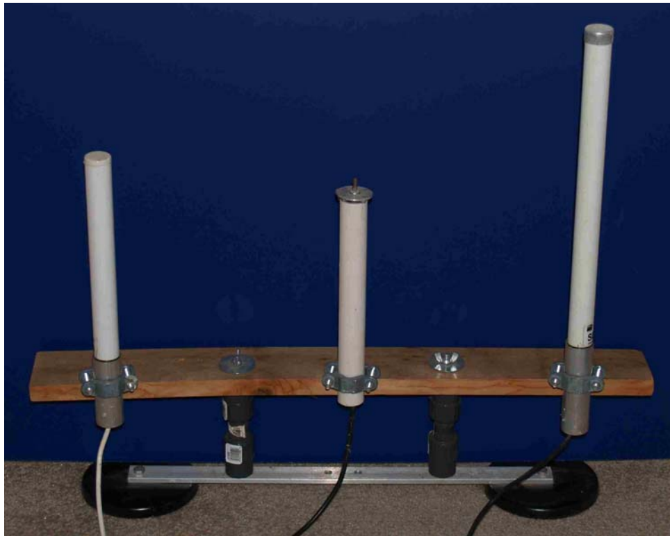
Figure 2 Antennas used for the 915-MHz, 2.4-GHz, and 5.8-GHz Bands
