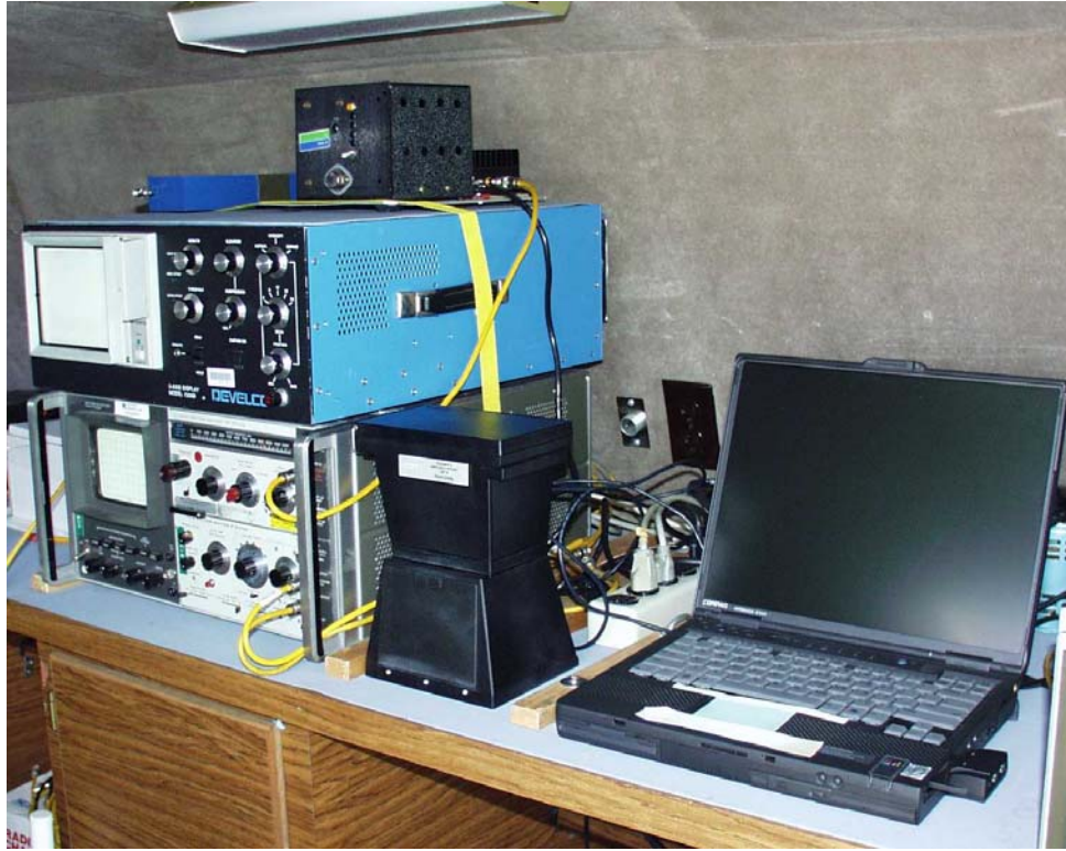
Figure 4 Instrumentation for the 0.1 to 1250 MHz Band
