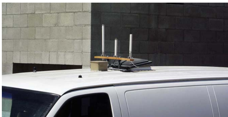
Figure 2 Photograph of Antennas on the Instrumentation Van
