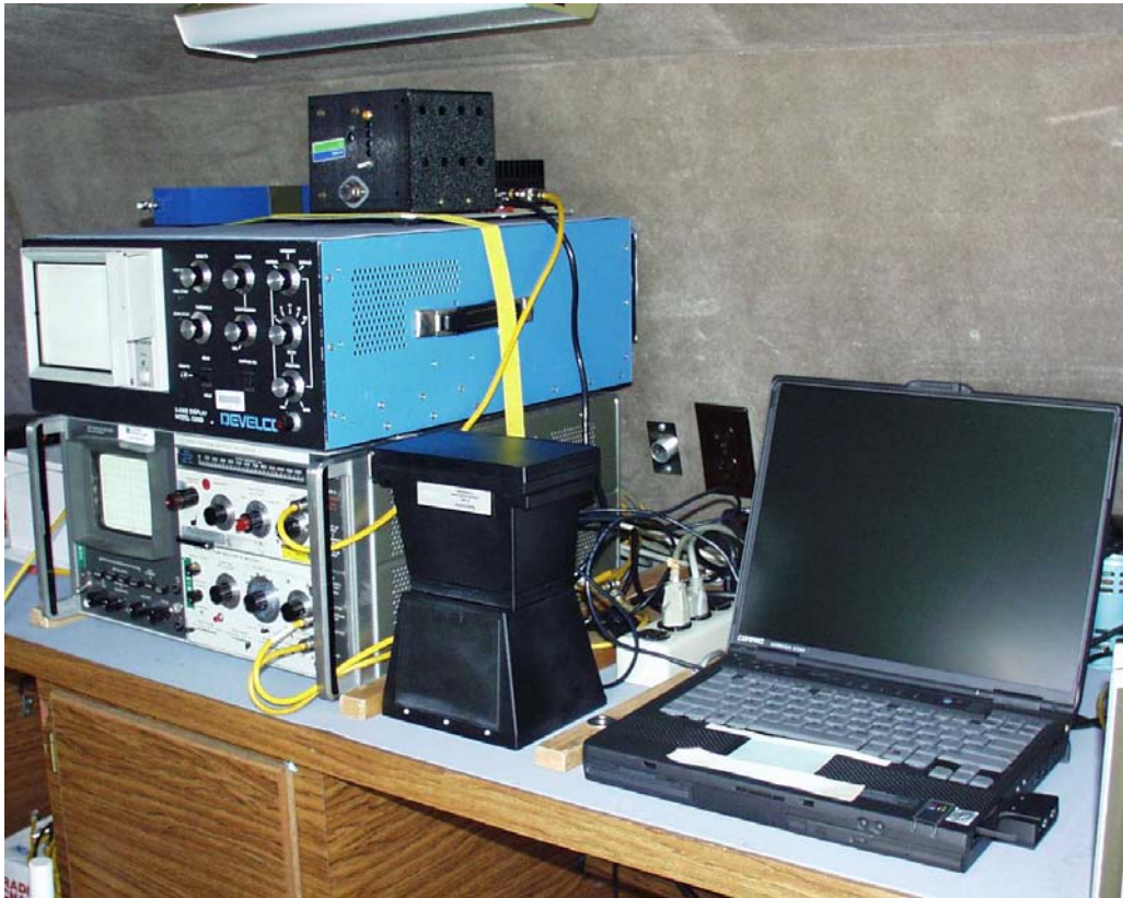
Figure 5 Instrumentation for the 0.1- to 1250-MHz Band
