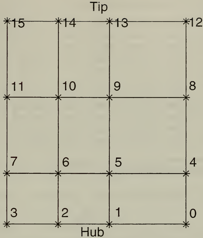
Figure 21. Control Point Numbering
