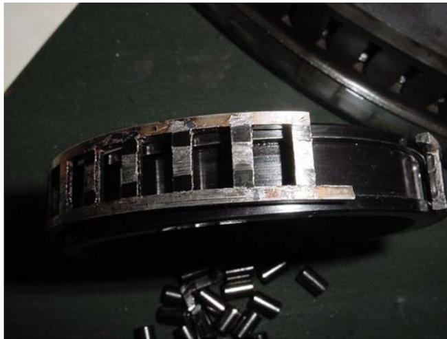
**Figure 1 - A failed roller bearing.**
