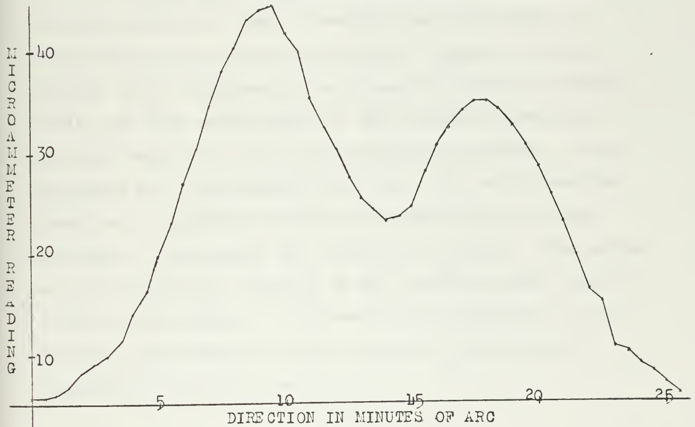
Fig. 4.2. Variation of microammeter reading with direction.
