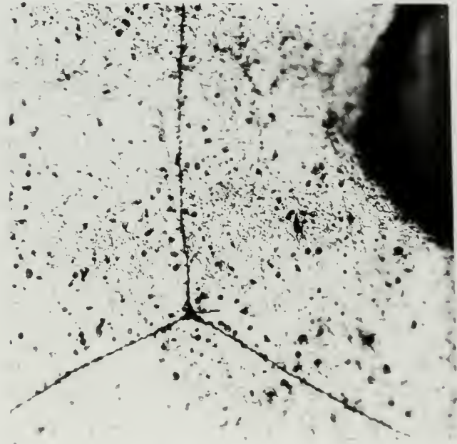
C. BOUNDARIES OF ALUMINUM TUBING, 500X
