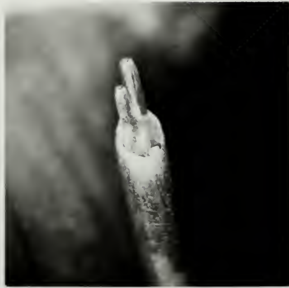
A. ALUMINUM TUBES NOT BONDED , VIEW A
