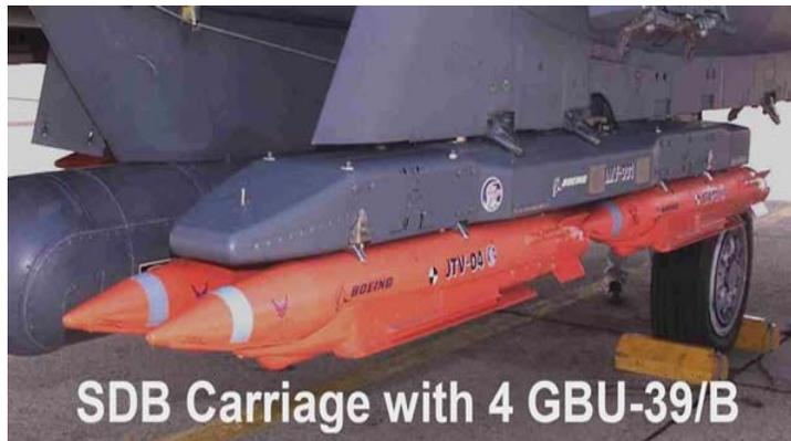
Figure 5 SDB carriage system (From Conventional Strike Weapon Presentation Dec 2003)
