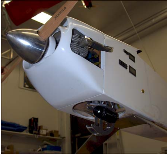
Figure 7. Gimbal detail in the Telemaster UAV.
