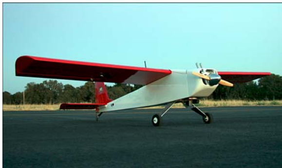
Figure 6. Modified Senior Telemaster UAV with gimballed camera.
