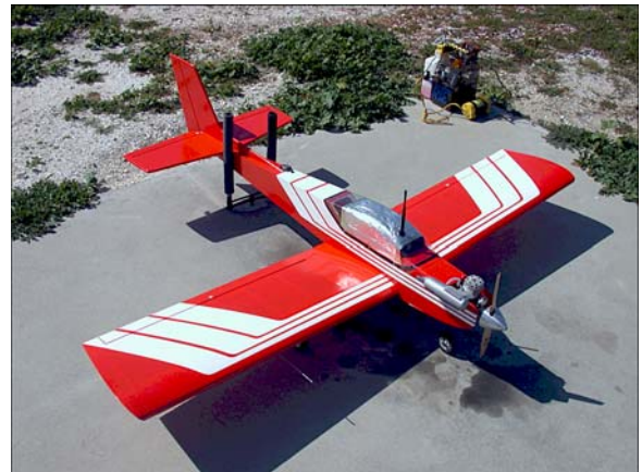
Figure 5. Tiger 60 ARF UAV fitted with Piccolo autopilot.
