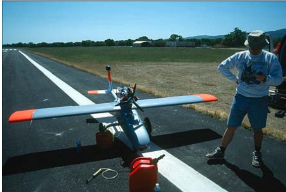
Figure 4. Tern UAV with Piccolo autopilot.
