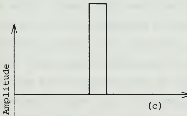
Figure 3.1. Autocorrelation of a complementary series.
